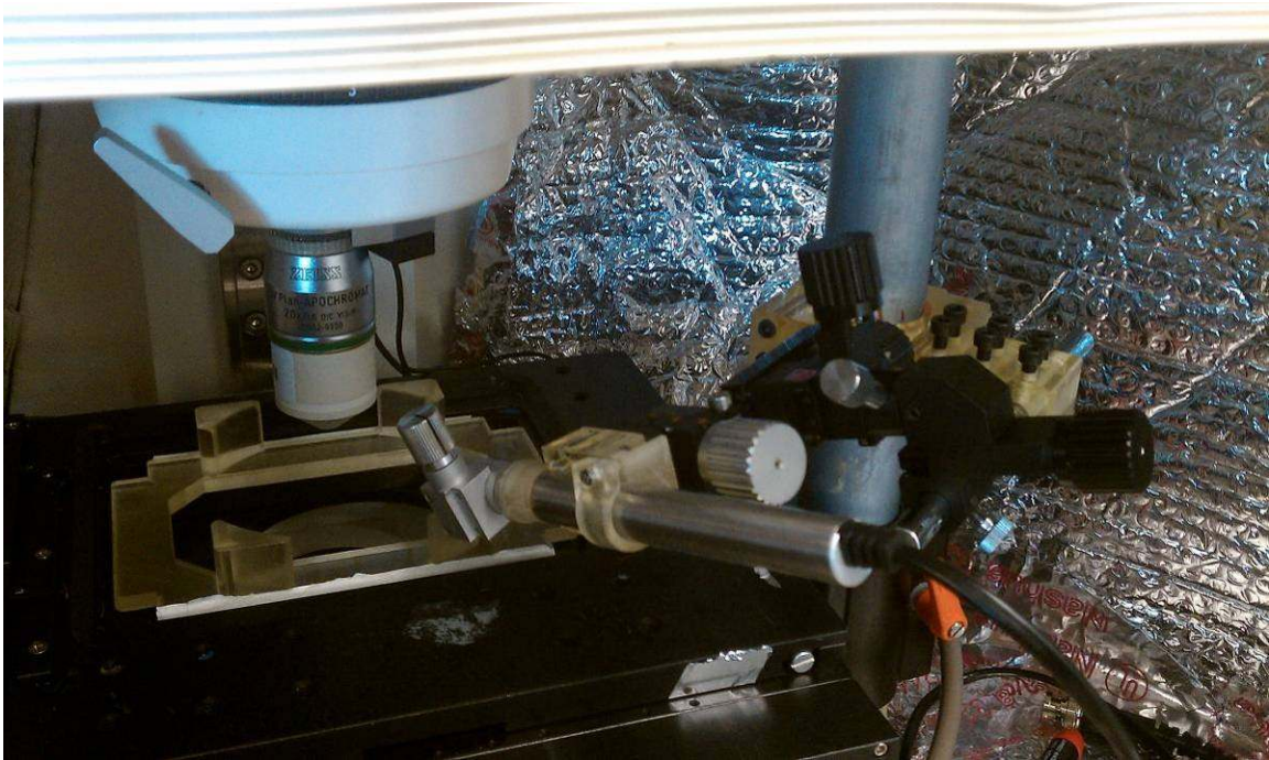
Figure 3.33: CAD drawing of the stand to secure the Narishige stage to a 2" OD post (top), and a photograph of the manual-stage-mounted mechanical controller and linear actuator in the neuronal calcium imaging station (bottom). This stand allows for coarse height, lateral, and rotational (around the post) adjustment. In the bottom picture, a custom built chuck for loading the cell culture systems can be seen below the microscope objective.
